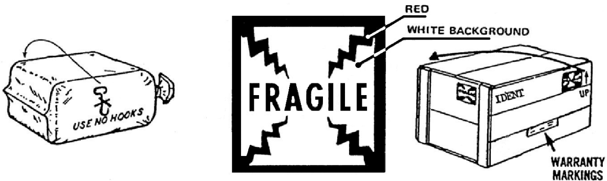
FIGURE 29. Examples of special marking (FRAGILE, UP, arrows, USE NO HOOKS and warranty marking).
